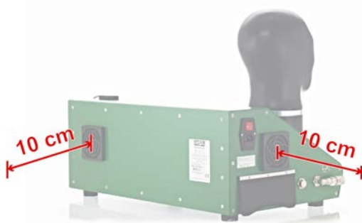
Fig. 8 Minimumsavstander for SmartCHECK basic
