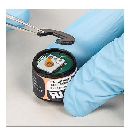
Carefully remove cell assembly by prying under the edge near the three connector pins
