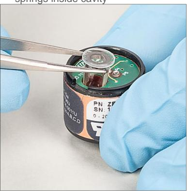
Apply light pressure with swab to seat fully in housing
