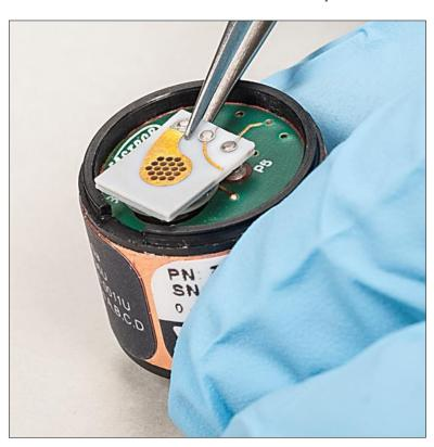
Replace the spacer surrounding the cell assembly
