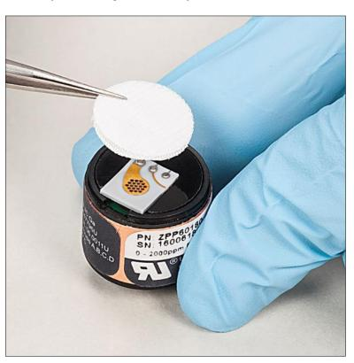
Align cap key with notch on housing and press down firmly to snap onto housing
