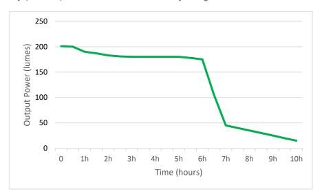
The enclosed diagram is indicative. Performance (output power, burn time) may vary depending on temperature and battery service life. Measurements are made at an ambient temperature of 20°C.
