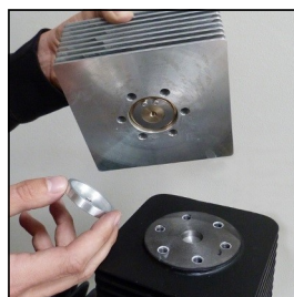
Fig. 2 - Remove lower valve gasket
