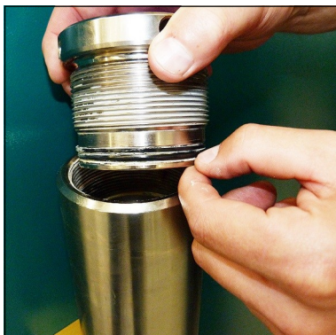
Fig. 2 - Change o-ring and back-up rings
