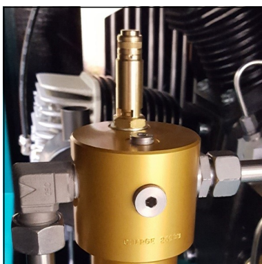
Safety valve 1st stage
