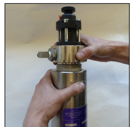
Fig. 3 - Open pre-filter cover
