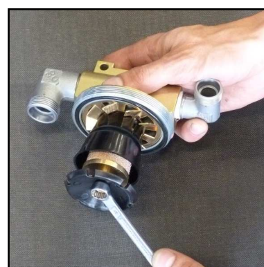
Fig. 2 - Loosen nut at the separator top
