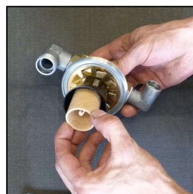
Fig. 3 - Change sinter filter
