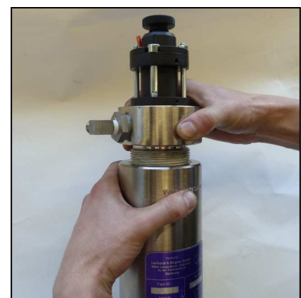
Fig. 3 - Open pre-filter cover
