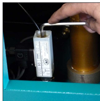
Final pressure switch
