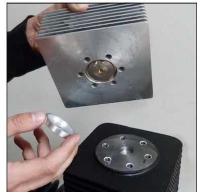
Fig. 2 - Remove lower valve gasket
