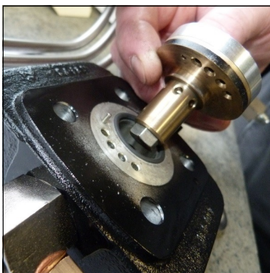
Fig. 1 - Ensure correct valve position (centre pin)
