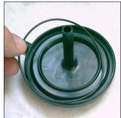
Fig. 3 - Place o-ring into the filter housing
