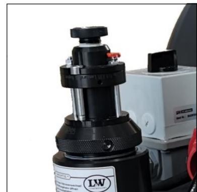
Safety valve 3rd stage
