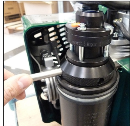
Fig. 1 -Loosen filter housing cover by using the filter tool
