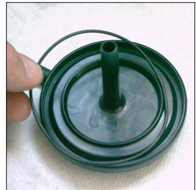
Fig. 3 - Place o-ring into the filter housing
