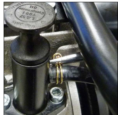
Fig. 9 - Fix spring wire clamp
