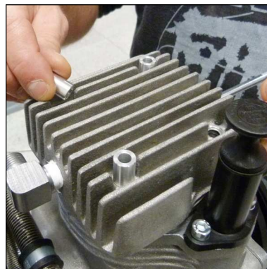
Fig. 8 - Place spacing sleeves
