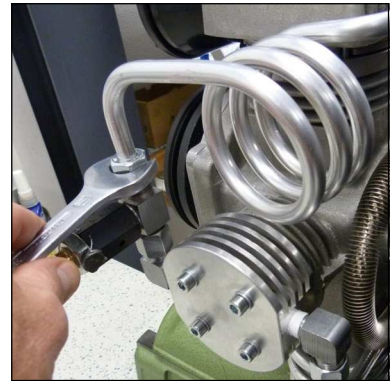
Fig. 1 - Loosen pipe connections
