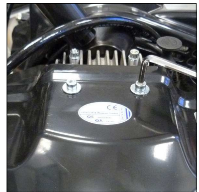
Fig. 1 - Loosen mounting screws of the fan protection cover
