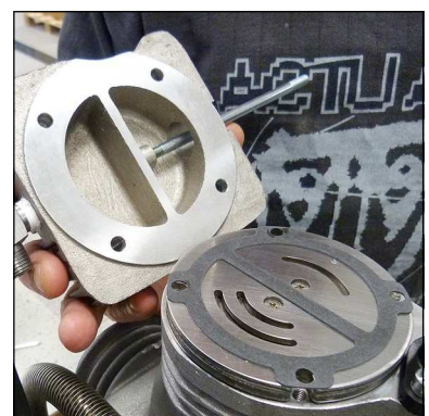
Fig. 4 - Remove valve head
