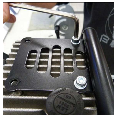
Fig. 3 - Loosen valve head screws
