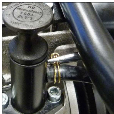
Fig. 2 - Remove spring wire clamp
