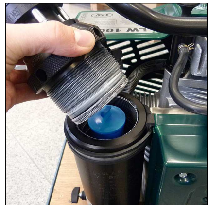
Fig. 2 - Remove filter housing cover
