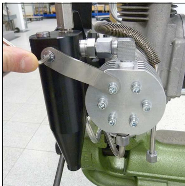
Fig. 1 - Loosen mounting screws
