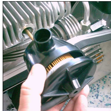
Fig. 2 - Pull out filter housing carefully
