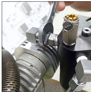
Fig. 2 - Loosen pipe connections
