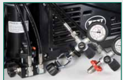
200/300 bar switch over device
