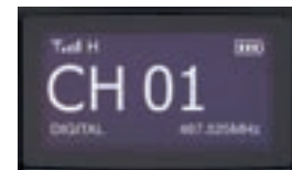
Informative display on UHF model shows both the channel number and the frequency
