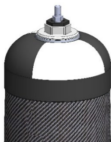
Figure 4: Cylinder with bicycle-type valve and internal pressure
