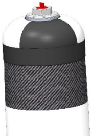
Figure 6: Cylinder with cap and without internal pressure
