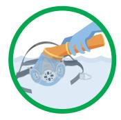
To remove debris and soil, manually clean the facepiece by immersing it in warm water with neutral detergent, scrub with soft brush until clean. Rinse thoroughly with fresh warm water.
